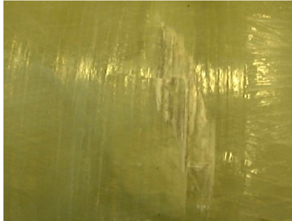
Figure 3a — Impact damage in combination with delamination and surface defects – not acceptable
