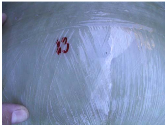
Figure 2 — Damage from abrasion and cuts— not accepted
