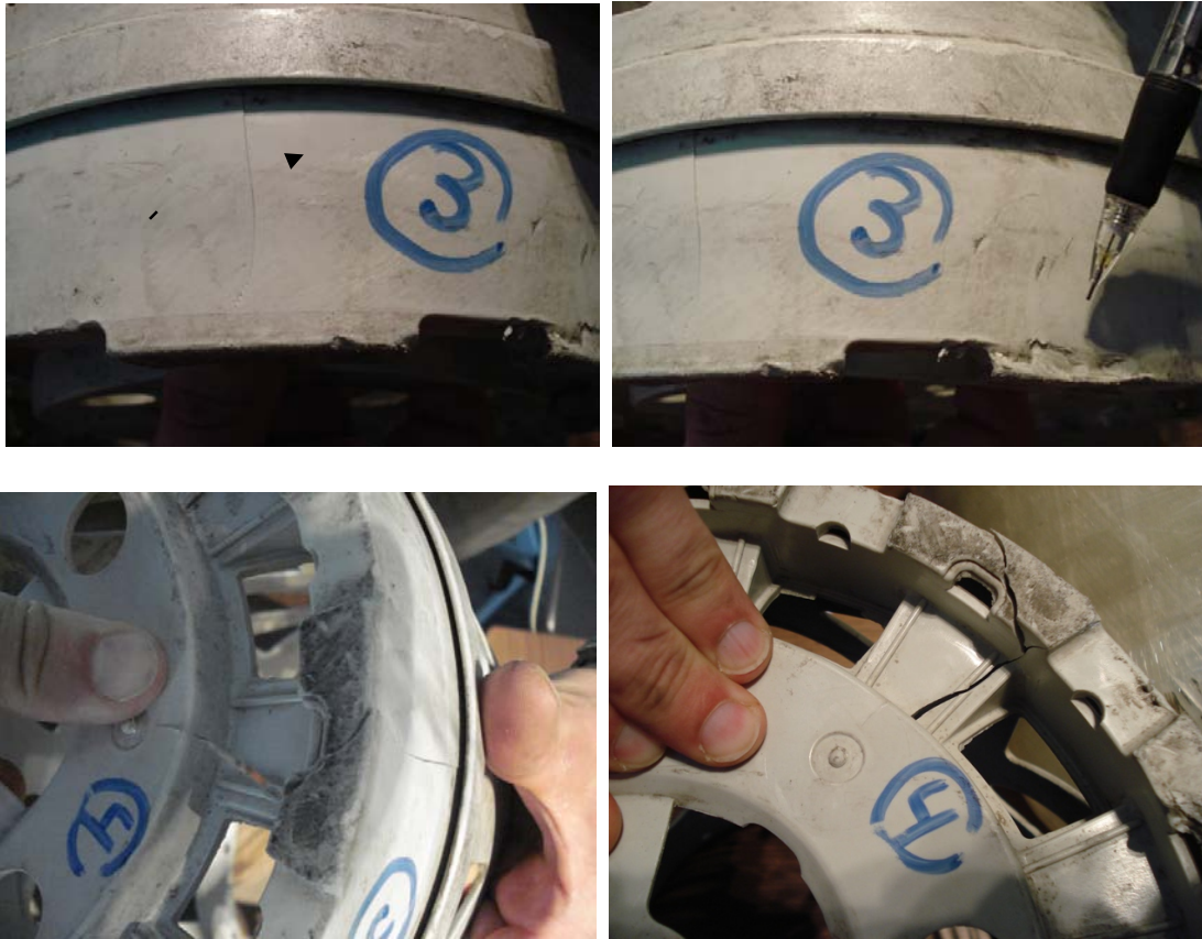
Figure 1b — Damage on casing base – not acceptable
