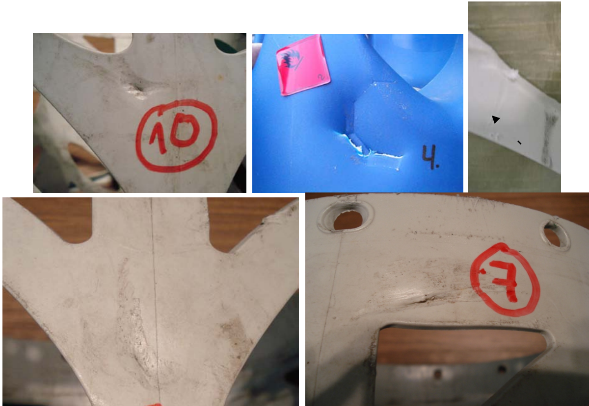
Figure 1c — Damage on casing cylindrical area – not acceptable
