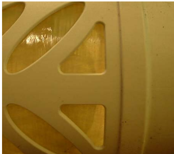
Figure 3b — Delamination and no surface damage - acceptable
