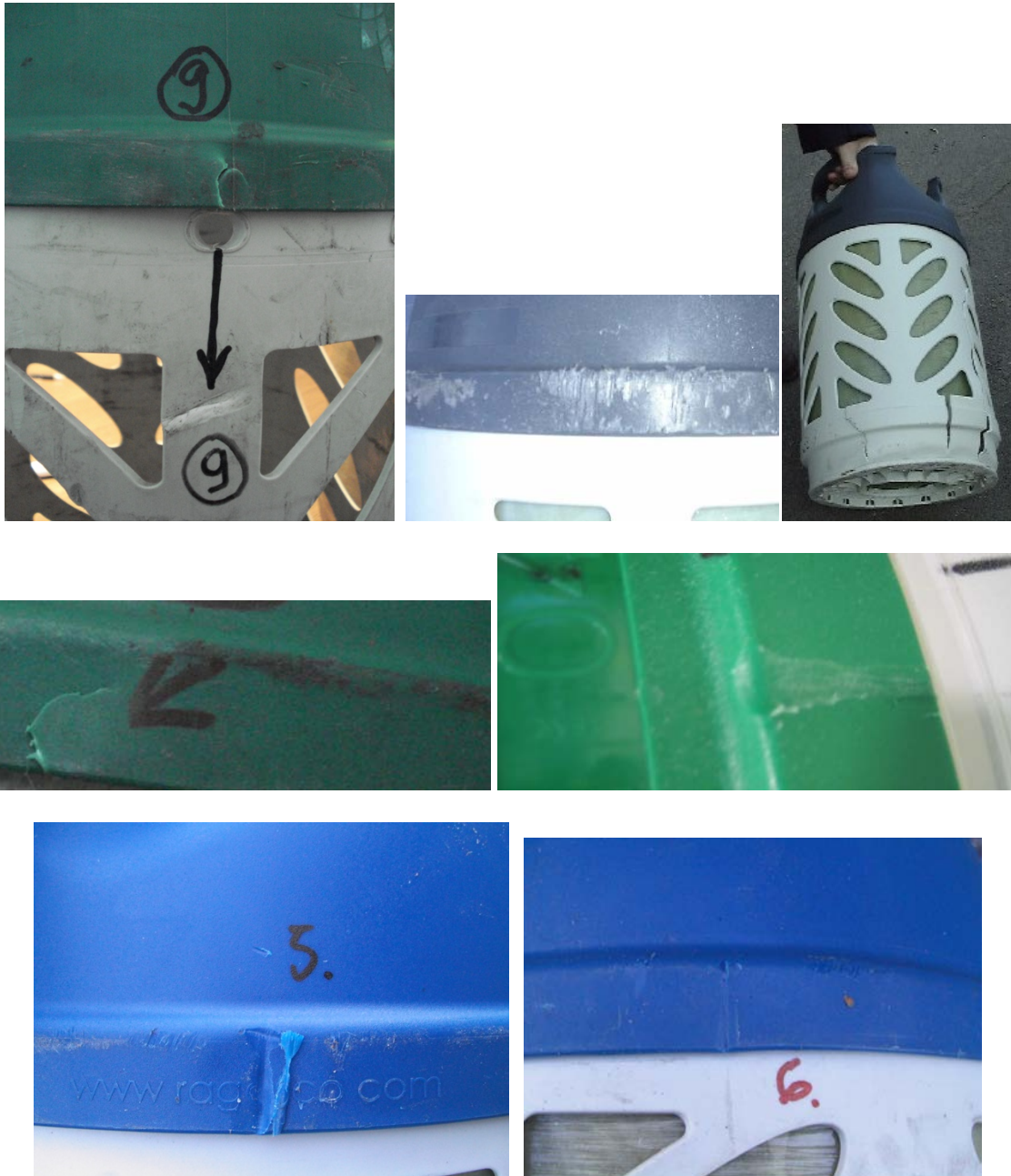
Figure 1a — Damage on casing “skirt”— not acceptable
