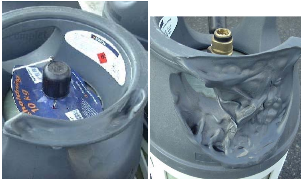
Figure 4 — Heat damage. This type of damage is not acceptable in any form
