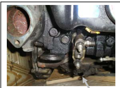
4.248 smaller injectors installed parallel to valve cover
